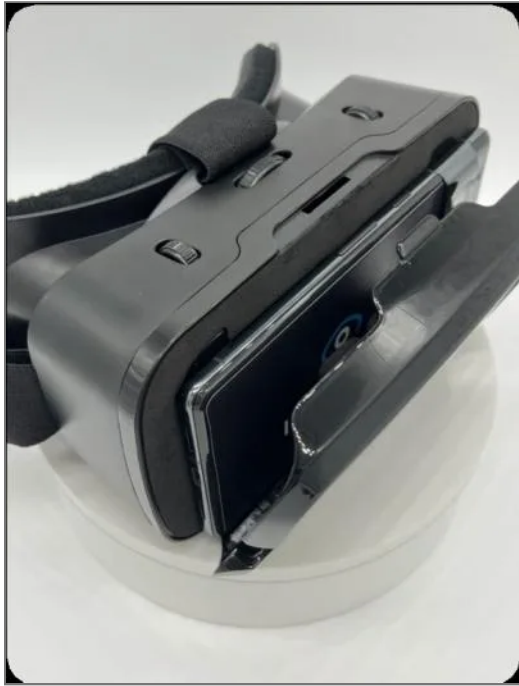
Removing the Vista display unit from the headset
