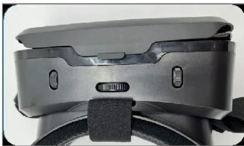
Vista headset — IPD dial in the center and focus wheels above each lens
